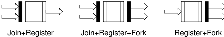
Figure 9.16: Schematic symbols for a handshake register fused with a Join and/or a Fork.
